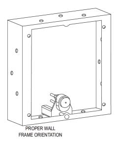
† Position of Sensor Box can be raised or lowered 1" (25 mm) if in conflict with Handicap Grab Bars.
